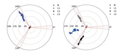
Figure 5: Eneida Feeder Current Imbalance Polar Plot for Old Slade Lane
