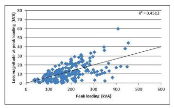
Figure 4: Correlation of Losses at Peak Loading with Peak Loading
