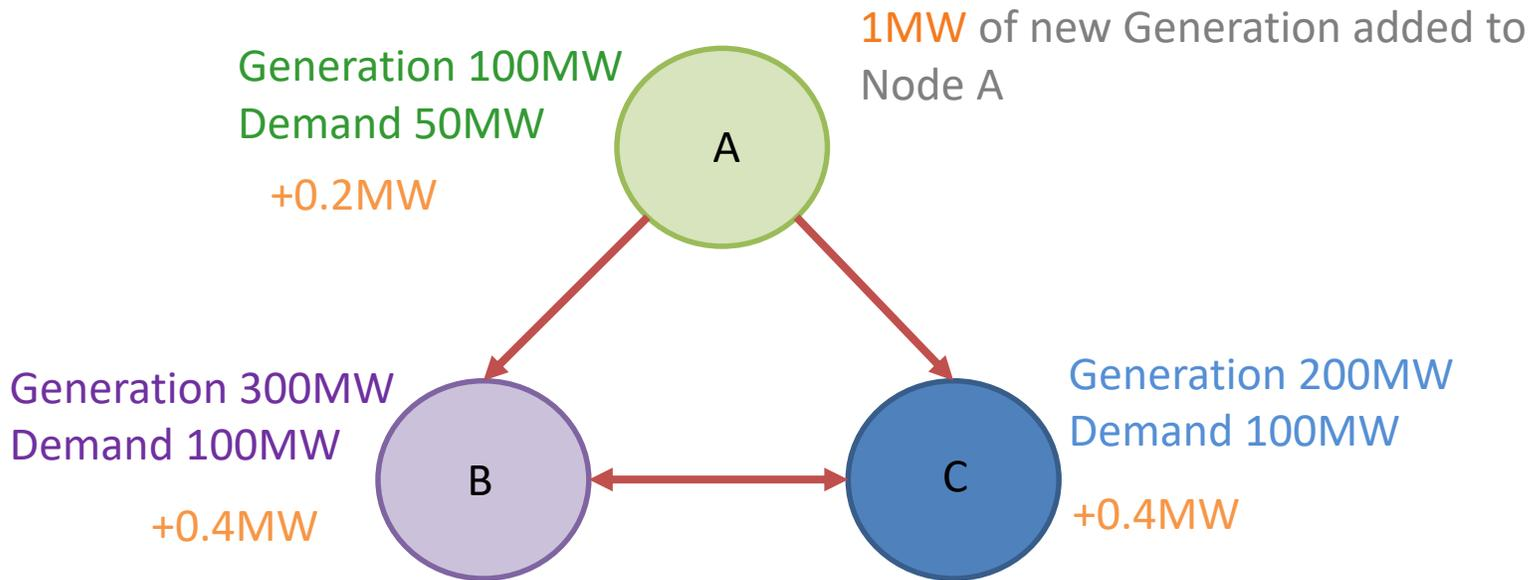
1MW of generation capacity is added to a node on the network. As the system has to be in balance, 1MW of demand has to be added too.
