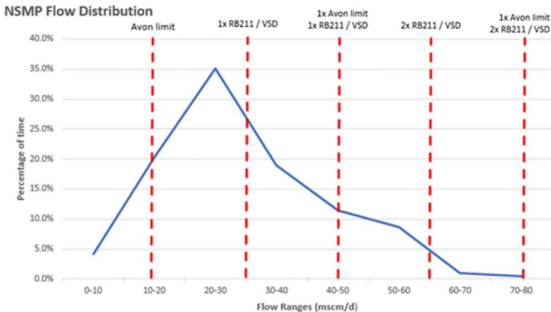
Figure 4 – Historical flow profile at St Fergus with associated compressor configurations
