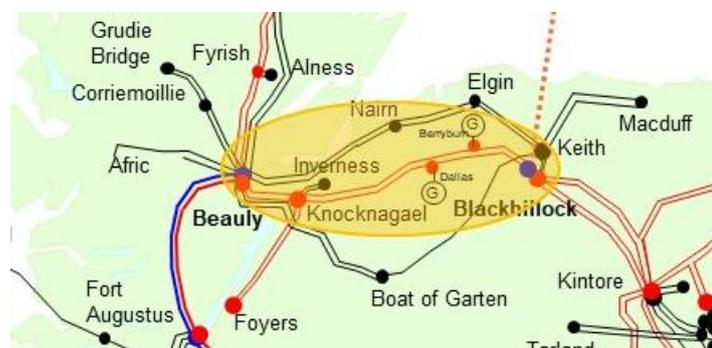
Reinforcement work has taken place on the overhead line between Beaulay and Blackhillock (B-B), over a relatively short period from 2009 to 2018, as a result of (i) required load driven reinforcement, (ii) new renewable generator connections.
