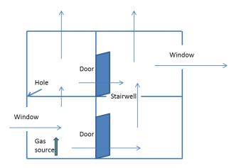
Figure D.2 Conceptual design for the gas migration experiment
