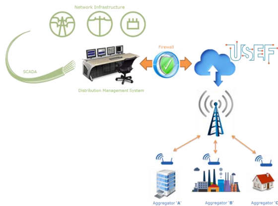
Figure 3: FUSION - Principle Architecture of the East Fife pilot
