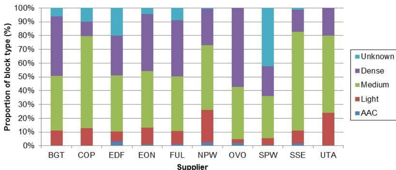
The distribution of concrete block densities was broadly similar across each supplier. Although there were a significant number of records from SPW which did not specify the density of concrete block used in the construction (listed as ‘Unknown’ in Figure 4), judging by their thermal conductivities the majority of these match dense concrete.
