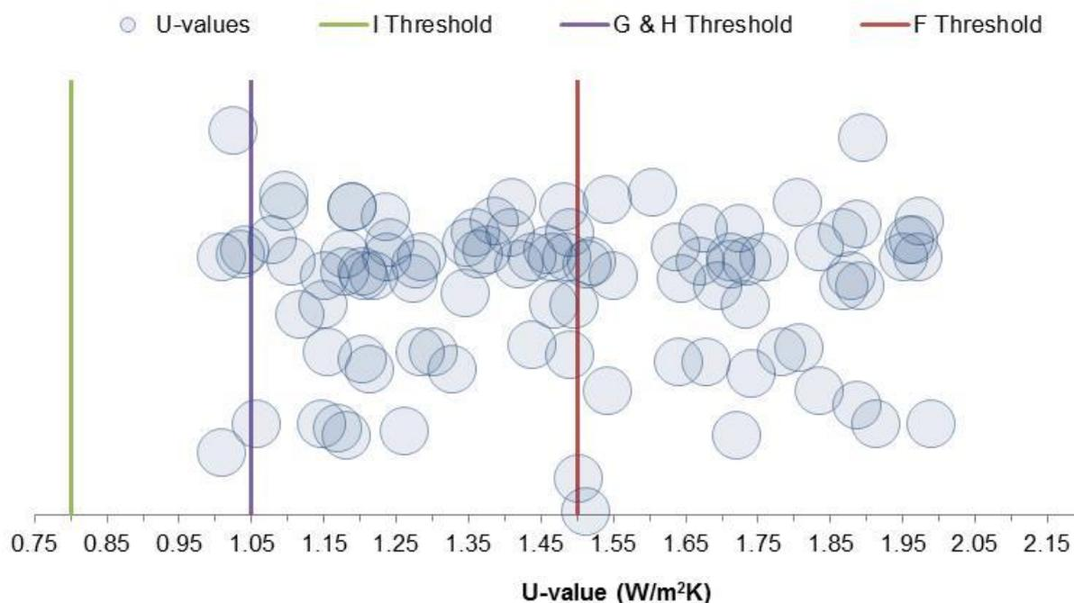
As a result, the U-values in the Evidence Audit dataset are lower than those seen in the Calculation Audit dataset. This could mean that since June 2016, assessors are reporting lower U-values than in reality in order to avoid having to provide additional evidence. Or, conversely, this could mean that prior to June 2016 when more rigorous evidence was not required, assessors were not calculating U-values correctly.
