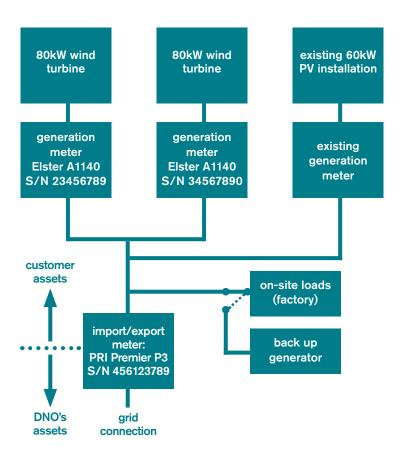
Also shown is an onsite load (a factory). The factory has a standby generator and interlocking is in place, and clearly indicated, to make sure that the standby generator cannot add to the generation or export meter readings.
