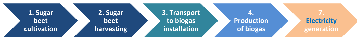
Figure 7: Example of a crop to electricity generation fuel chain through the production of biogas: sugar beet (KEY: Dark blue: Cultivation and harvesting, Teal: Transport and distribution, Blue: Processing, Orange: electricity generation.)
