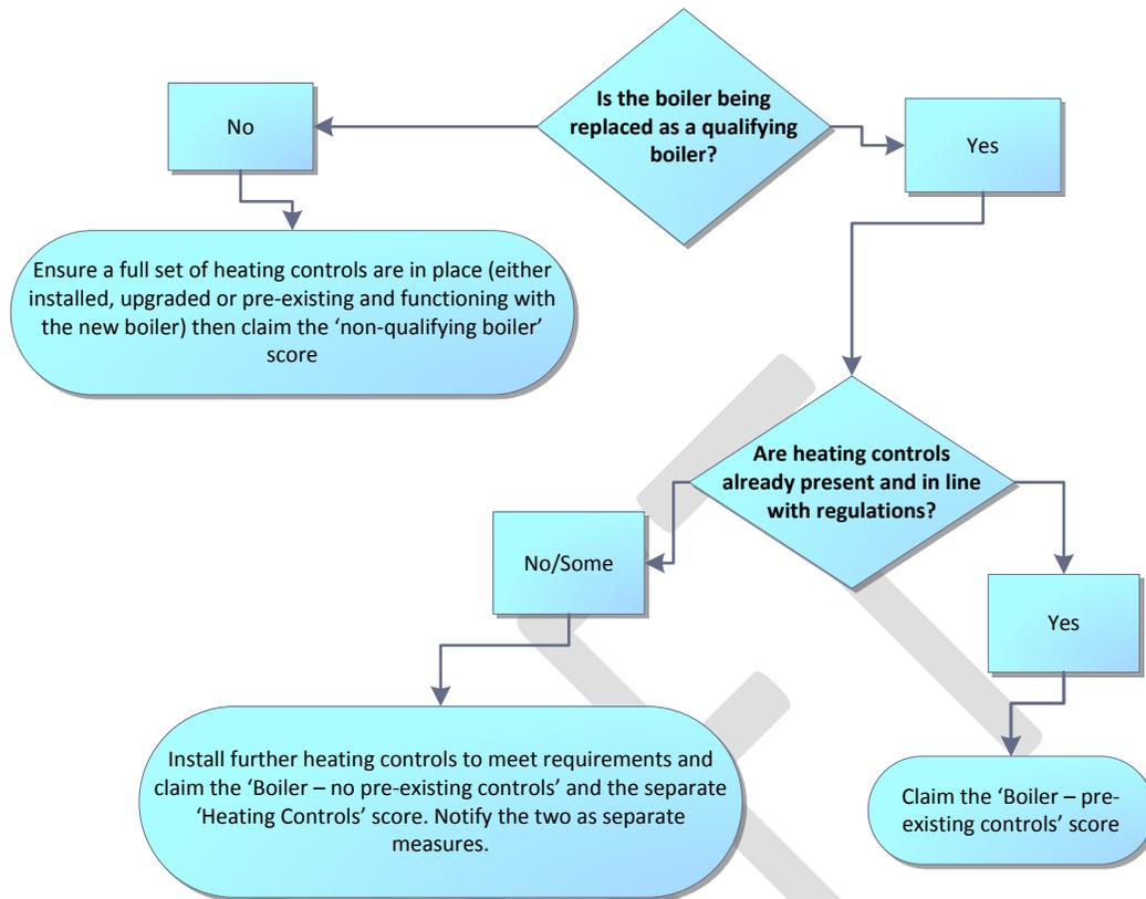
**Figure 3** Flowchart for selecting boiler and heating controls scores
