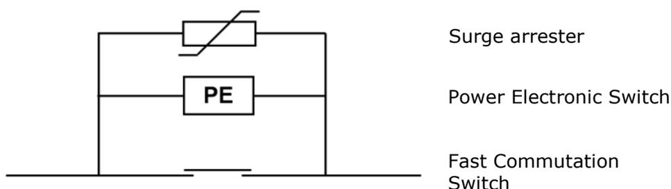
Figure 4 - Principle layout of the FLCB.
