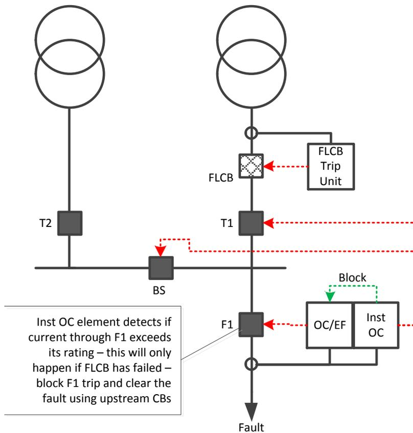
Figure 12 - Independent backup protection option 3 - Ultra-Fast Earth Switch
