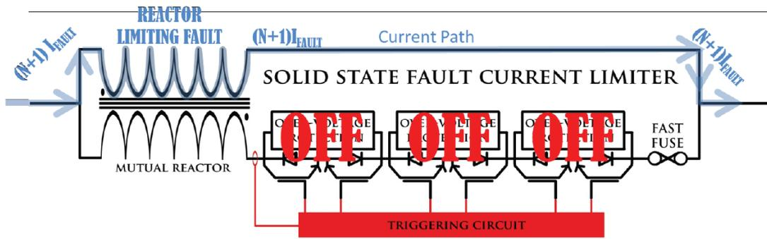
Figure 14: SSFCL reactor limiting the Fault Current
