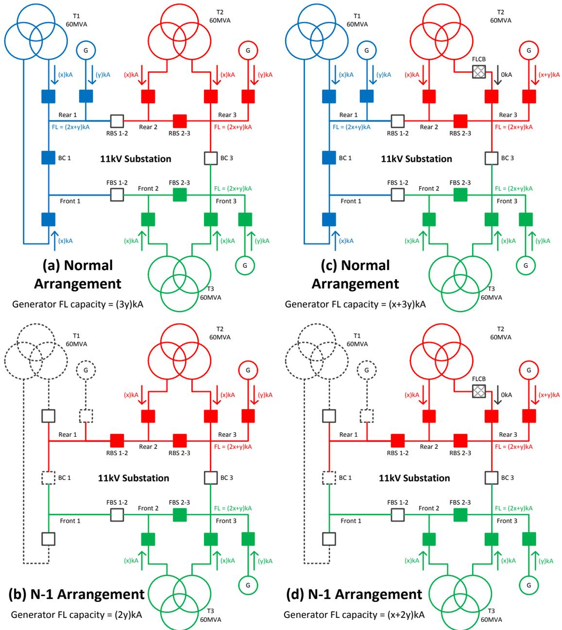
Figure 9 - Operating scenarios for a 3x60MVA substation, with/without a FLCB. NB FLCB isolation/bypass CBs are omitted for clarity
