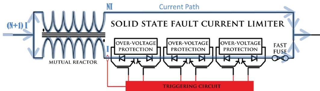
Figure 13: SSFCL sharing current: in the normal condition the mutual reactor has zero reactance
