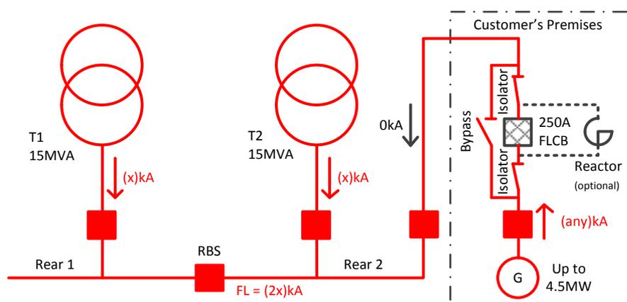
Figure 18 - Schematic diagram of Method 2 trial
