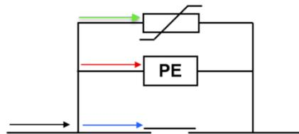
Figure 5 - Line current and currents through the mechanical switch and the power electronic switch and the surge arrester.
