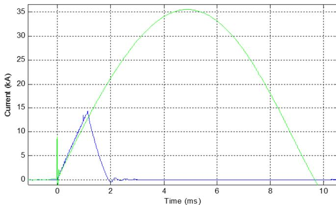
Figure 7 - Measured prospective and limited short circuit currents during high power testing.
