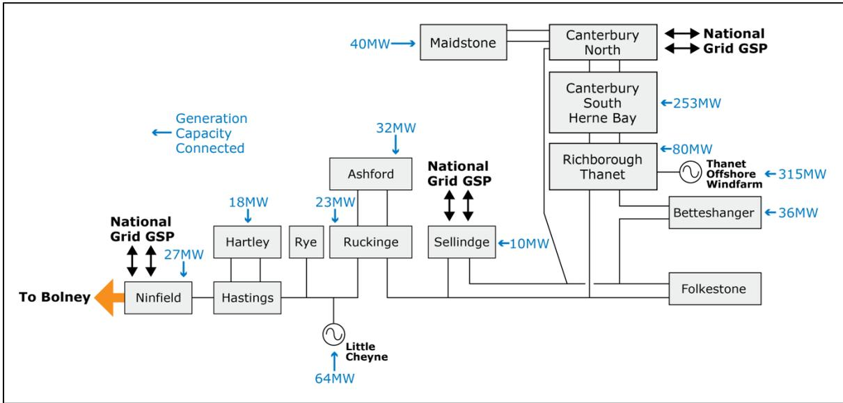
**Figure A3.5** Simplified diagram of 132kV UKPN network Ninfield to Canterbury
