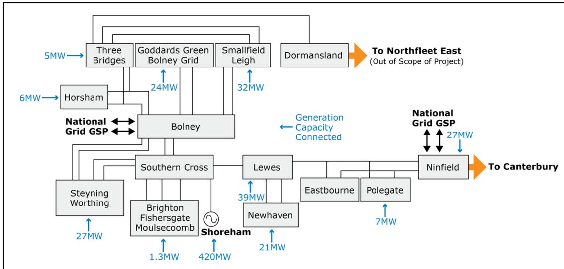
**Figure A3.4** Simplified diagram of 132kV UKPN network Bolney to Ninfield
