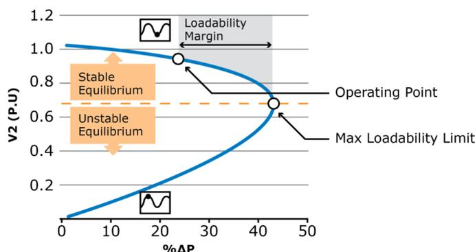
**Figure A6.1** P-V curve (Moeller & Poeller, 2016)
