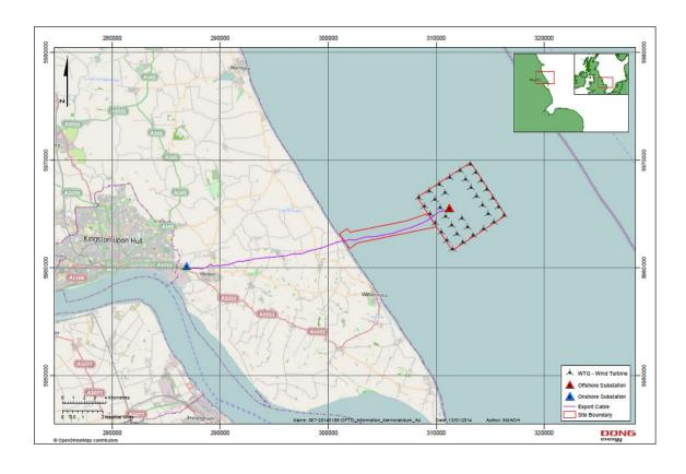
$<sup>^3</sup>$  The maximum possible output of the windfarm is 210MW at the offshore platform. A maximum output of 205MW is allowed to be exported to the OFTO point of connection to the onshore system. The difference is attributed to array cable losses. See page 2 of the PIM
