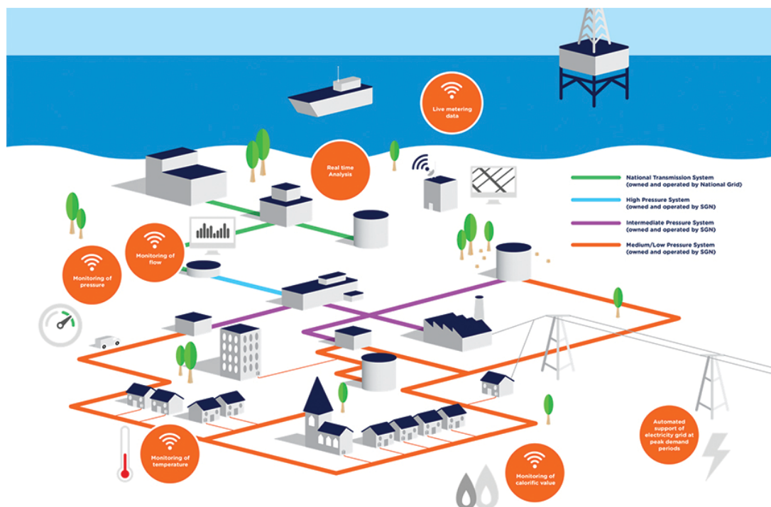
Fig 7.2 Beach to meter diagram
