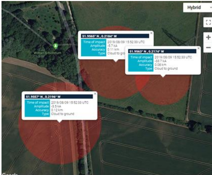
Figure 4 - Three simultaneous lightning strikes close to Willian Arboretum at 15:52hrs – Data Source: Meteogroup
