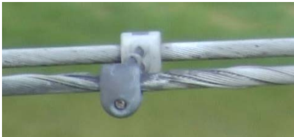
Figure 19: conductor damage at spacer clamping position at ZF Route.
