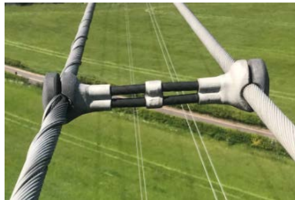
Figure 19: conductor damage at spacer clamping position at ZE Route.
