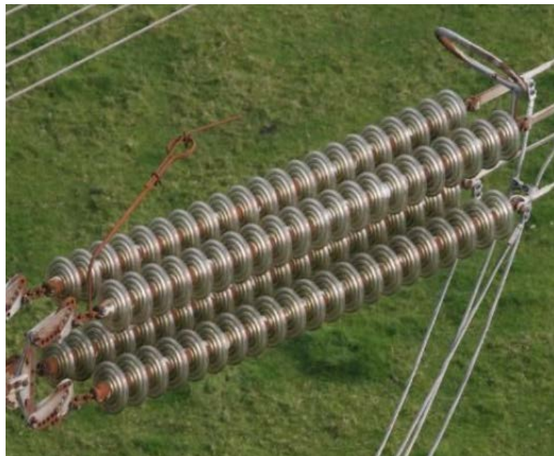
Figure 5: tension insulator severely rust and degraded mechanical caps at ZC(S) Route.
