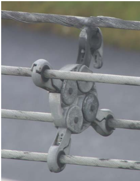
Figure 7: conductor damaged at 'Dunlop' spacer-damper clamping position at ZP Route (023-024).
