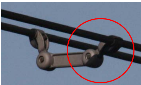
Figure 29: spacer-damper collapsed.
