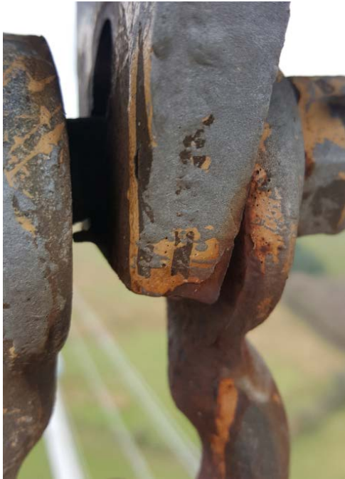
Figure 14: worn of suspension earth wire fitting at ZP051
