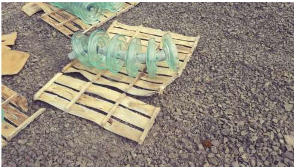
Figure 8: Carolina Port - Degraded Packaging of Stock Held Inside
