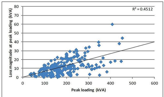
Figure 4: Correlation of Losses at Peak Loading with Peak Loading
