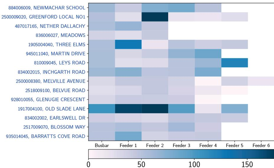
**Figure 3:** Color map where the color intensity corresponds to the imbalance value for each sds/feeder.
