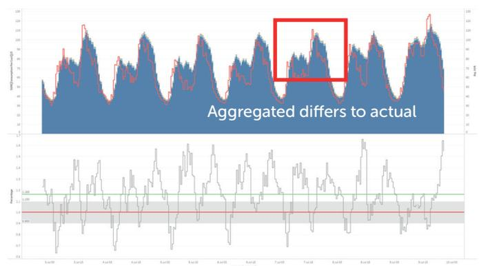
Figure 9: D0030 Aggregated Profile Shapes Vs LV Monitoring Data
