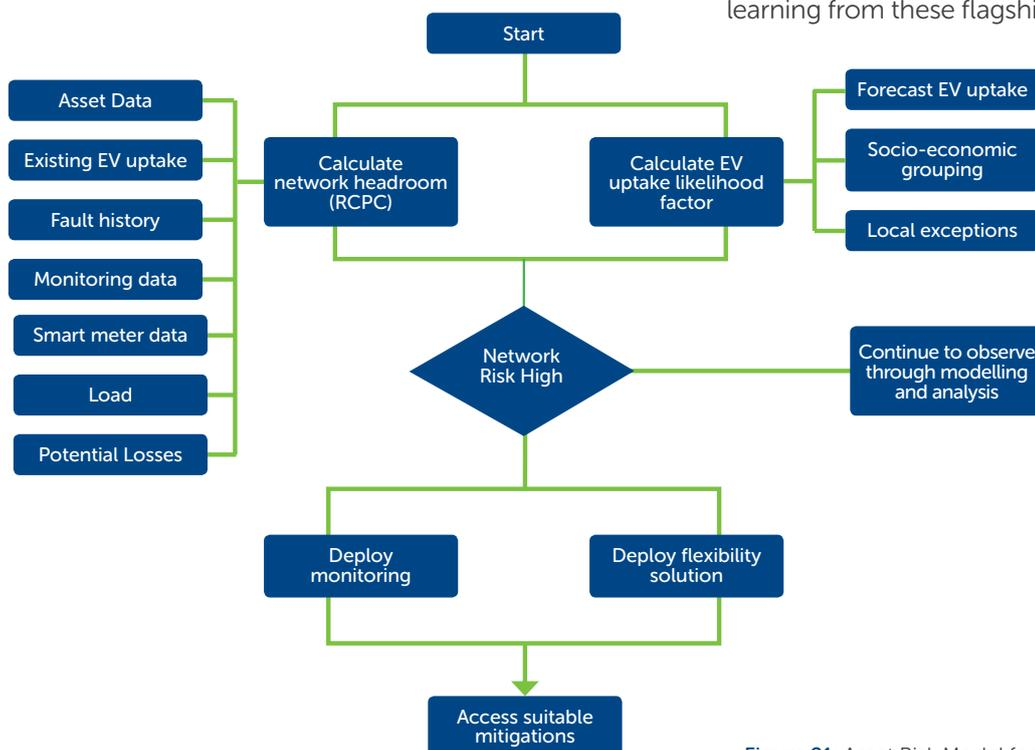
Figure 21: Asset Risk Model for deployment of monitoring equipment
