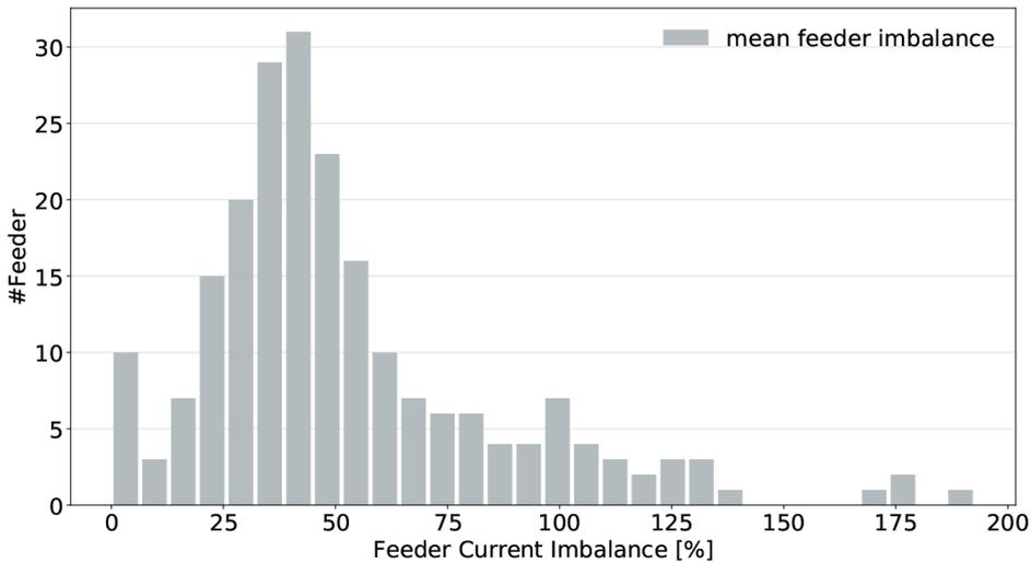
**Figure 2:** Distribution of Current Imbalance (x-axis) across the population of Feeders (y-axis). For each Feeder, the value of current imbalance is the aggregated mean value of current imbalance calculations over the period of reference (from 2019-04-02 23:59:00 to 2019-04-30 23:59:00). Current imbalance is being calculated as the ratio between the max deviation of the 3 phase currents from their mean value, and their mean value.
