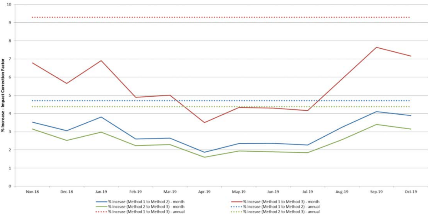
Figure B4: Average monthly (solid line) and annual (dotted line) energy cost correction factors for transitioning from methods '1 to 2' (blue line), '1 to 3' (red line), and '2 to 3' (green line). The annual numbers are equivalent to the annual correction factors, and in order of listing, these factors are 4.7%, 9.3% and 4.4%.
