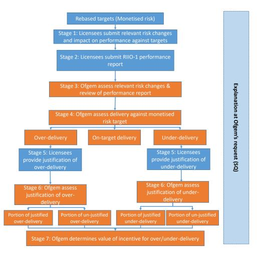
Figure 1: Process flow diagram for the NOMs incentive mechanism
