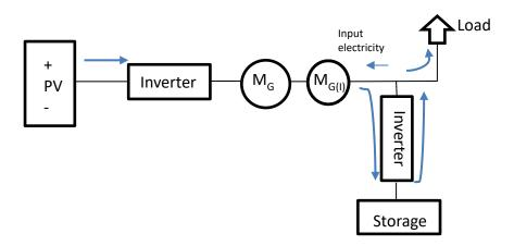
3.30. In this scenario, co-located storage has been installed on the site of the RO generating station to help meet the on-site demand load. The storage facility can only be charged by the electricity produced by the generating station. There is no grid interface.
