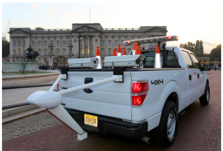
Figure 8 – Photograph of our Mobile Asset Assessment Vehicle in use
