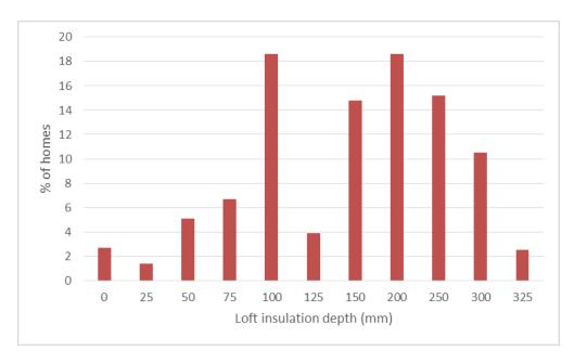
Figure 2: Distribution of loft insulation depths within England.
