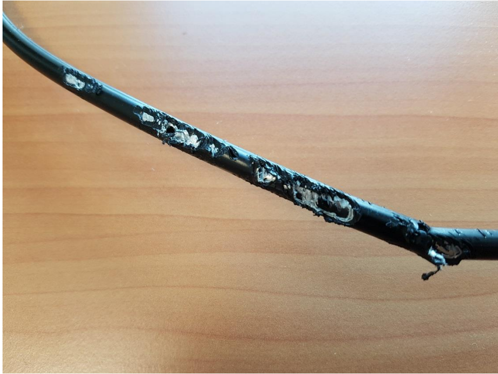
Animal damage to plastic coated mild steel sample line
