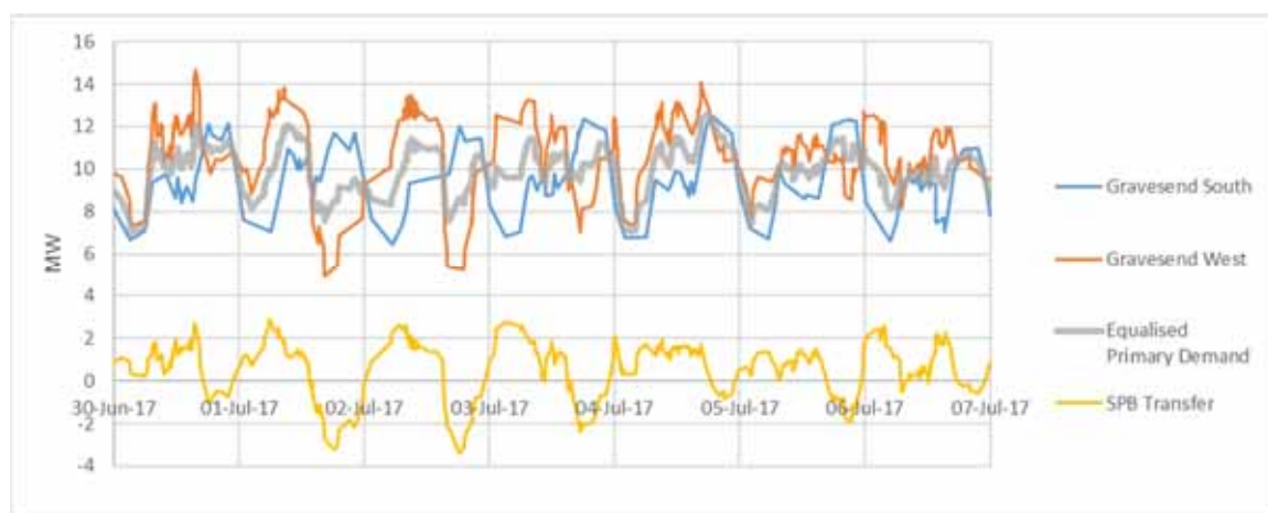
Figure 10.4.5. Demand at Gravesend South and Gravesend West Primaries during July 2017 and the estimated profile if an SPB were installed
