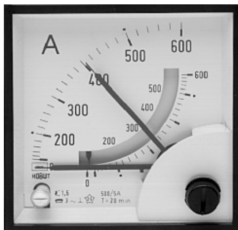
Figure 1. Conventional Maximum Demand Indicators (Source: HOBUT)
