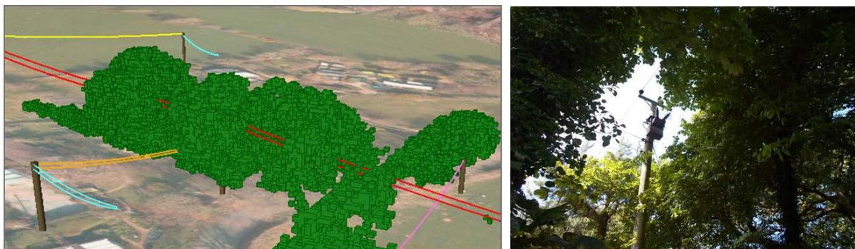
Figure 22 - Virtual World vs Real World Representation of a Vegetation Intrusion
