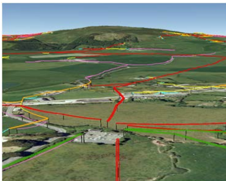
Figure 8 - Fugro ROAMES Virtual World OHL Network generated from Fixed Wing surveys
