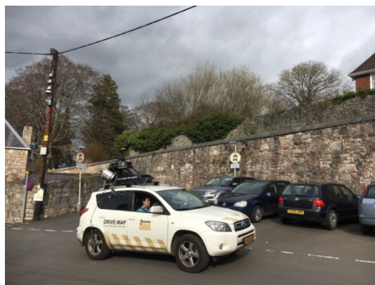
Figure 12 - Fugro Ground Based Survey of LV OHL Network in Ruthin
