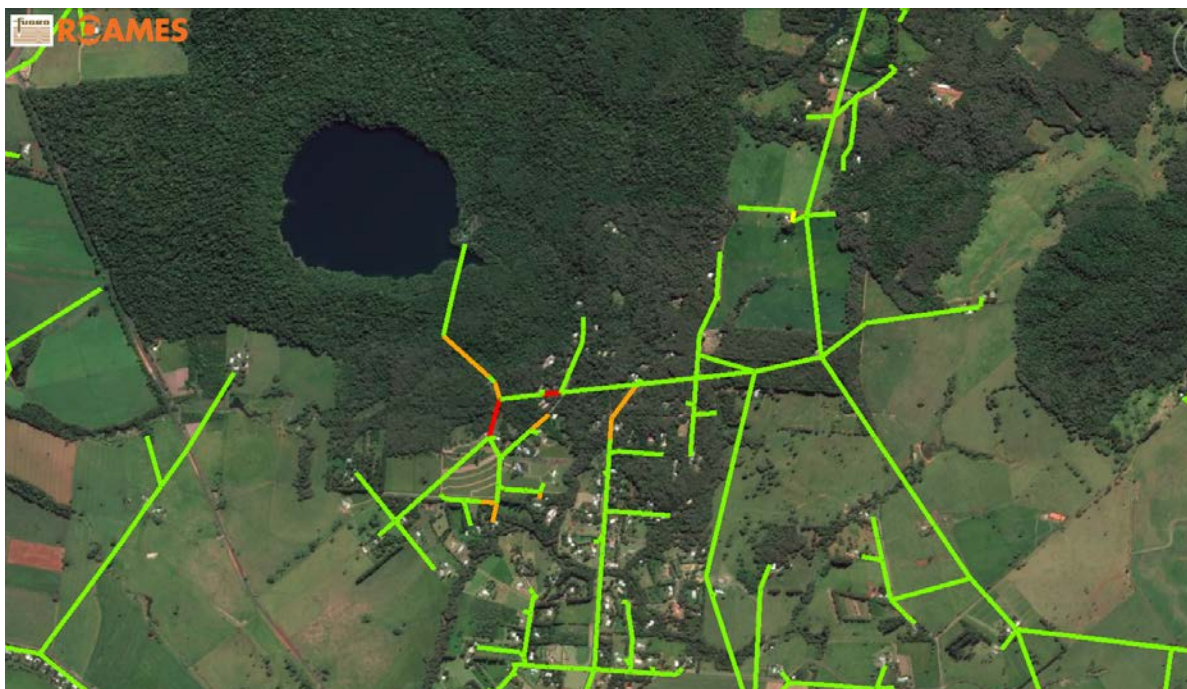
Figure C3: Example visualisation of heat-map showing vegetation growth rate at span level - red indicates area of high growth rate (based on client defined thresholds) transitioning to green indicating areas of low growth rate
