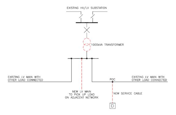
The RSN for the Reinforcement is the HV/LV transformer
