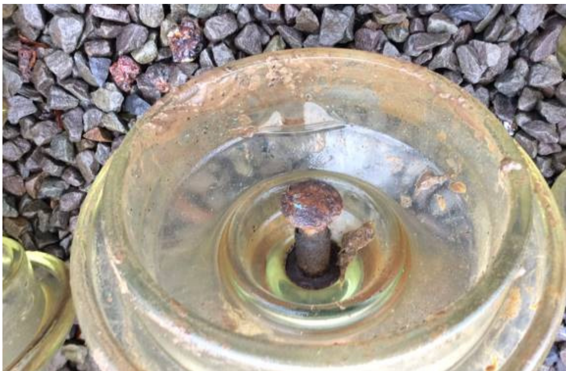
Photograph 2 - the metal pin of the glass insulator at the point of failure
