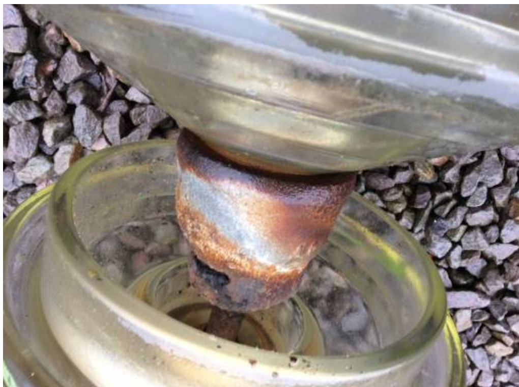
Photograph 1 - the metal cap of the glass insulator at the point of failure
