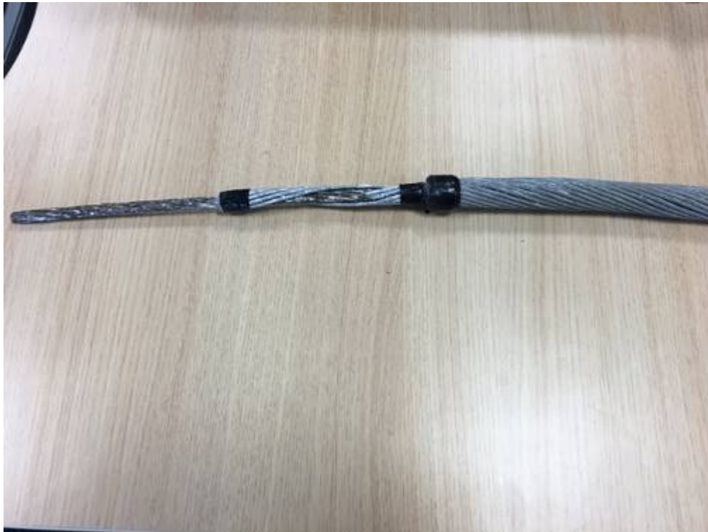
Photograph 3 - the corrosion within the failed earth wire
