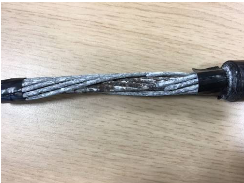
Photograph 4 - a close-up of the corrosion within the earth wire
