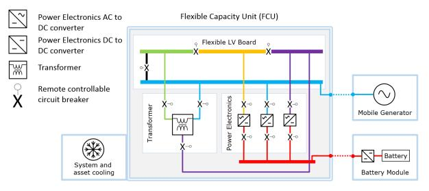
*Figure D.3: High level arrangement of a Flexible Capacity Unit (single line diagram to represent three phases)*
