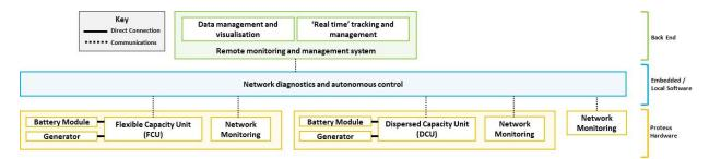
*Figure D.1: Components of the Temporary Solution enabled by Proteus*
