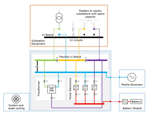
*Figure D.4: An example configuration of a FCU solution, using a 3-port SOP and a battery module (single line diagram to represent three phases)*
