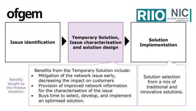
*Figure 2.2: Method for managing network capacity issues which is enabled by Proteus, and its benefits.*
