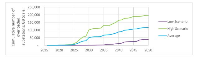
*Figure 3.1: The number of substations which are expected to be overloaded over Great Britain scale over the range of scenarios modelled*
