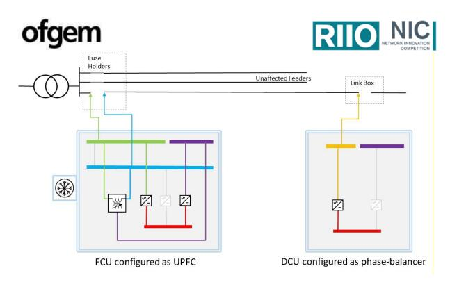
Figure D.7: Example Proteus installation – [Case Study 3]
