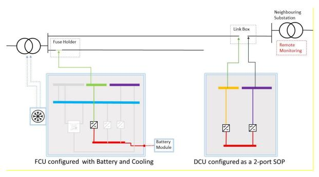
Figure D.5: Example Proteus installation – [Case Study 1]
