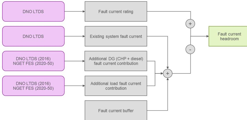
Figure 3 Schematic representation of data sources used to calculate fault current headroom
