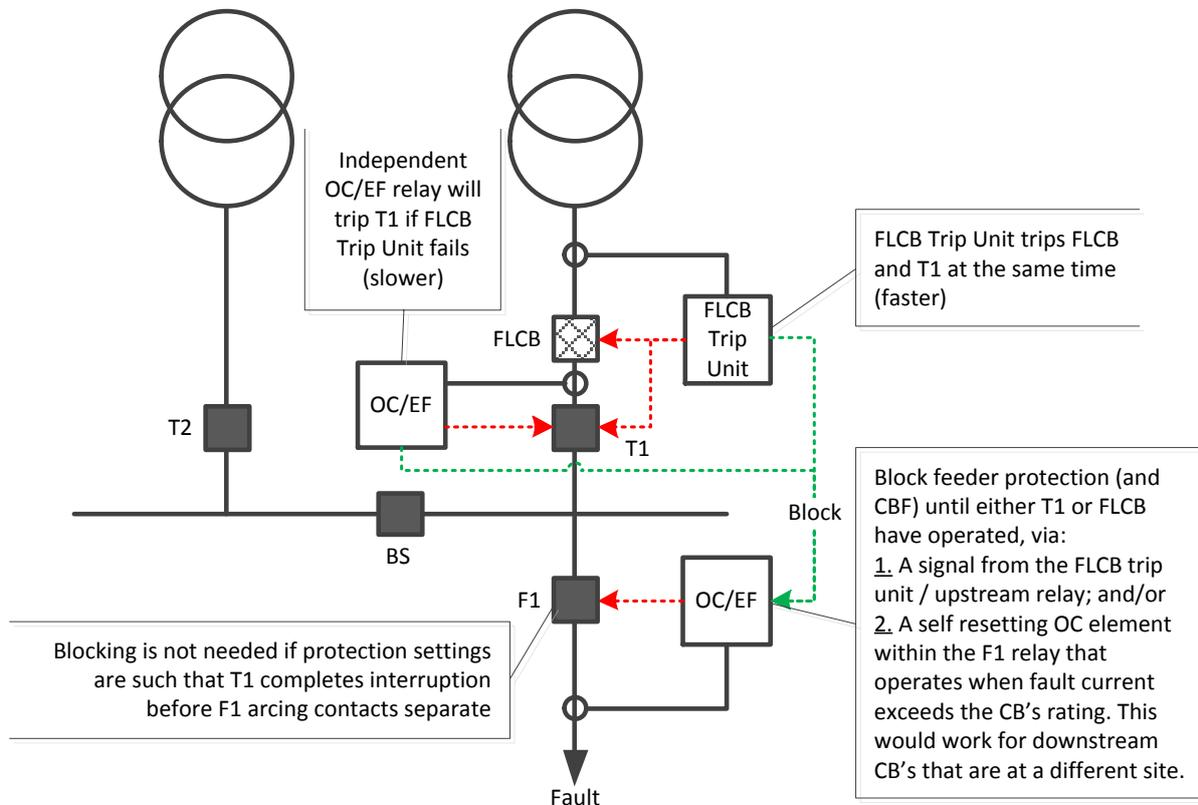
Figure 10 - Independent backup protection option 1 - Adaptive Protection
