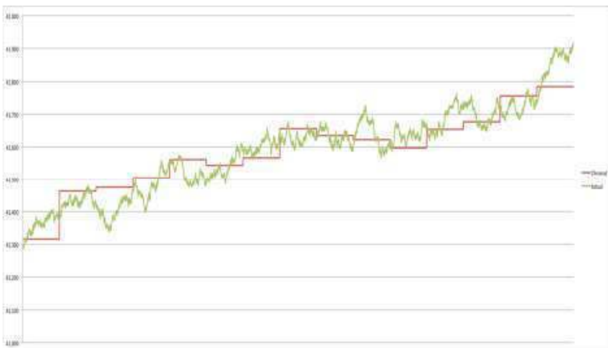
Figure 1: Plot showing actual CV of natural gas versus value reported by Danalyzer
