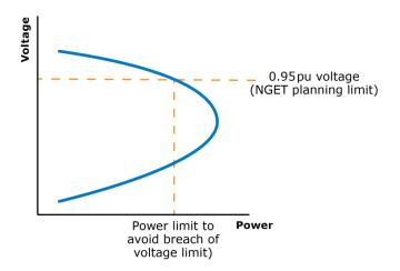
Figure A6.3 Example of P-V curve used by NGET (Moeller & Poeller, 2016)
