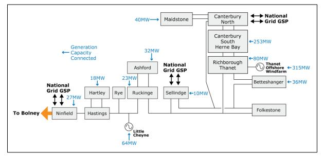
Figure A3.5 Simplified diagram of 132kV UKPN network Ninfield to Canterbury
