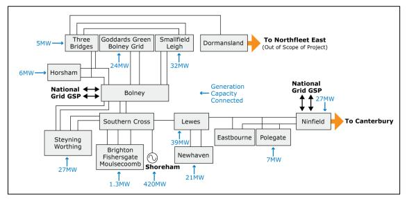
Figure A3.4 Simplified diagram of 132kV UKPN network Bolney to Ninfield
