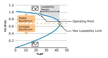
Figure A6.1 P-V curve (Moeller & Poeller, 2016)
