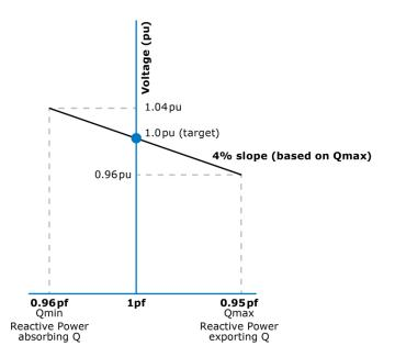
Figure A6.2 Voltage droop/slope approach in DERs (Moeller & Poeller, 2016)
