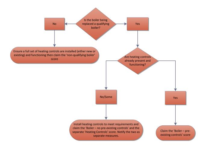
Figure 7: Flowchart for selecting boiler and heating controls scores (to be used in conjunction with Chapter 7.7)
