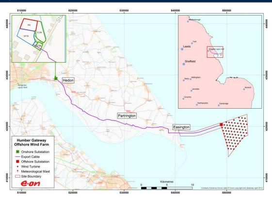
Figure 1 - Location of the HG Offshore Wind Farm and Transmission Assets
