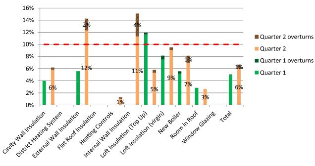
Fig. 3) Installation failure rates as a percentage of all monitored measures per measure category
