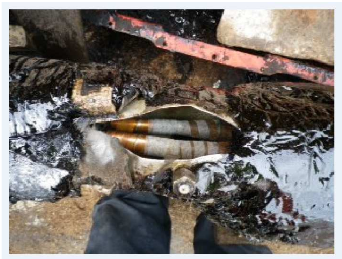
Photograph 2 – The ruptured casing of the failed joint of the 33kV fluid-filled cable
