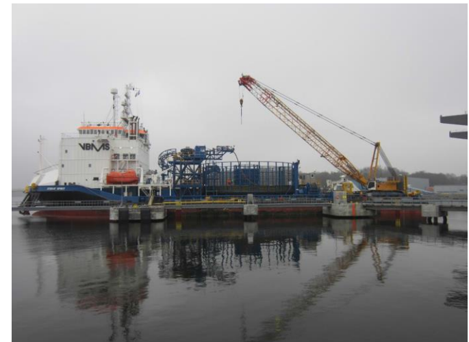
Stemat Spirit loading of offshore export cables.
