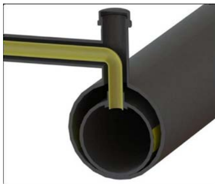
Figure 3 - A new PE main inserted within a parent metallic main with the service reconnected
