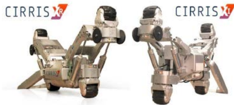
Figure 1 – CIRRIS XR™ - The Repair Robot (Left), CIRRIS XI™ - The Inspection Robot (Right)
