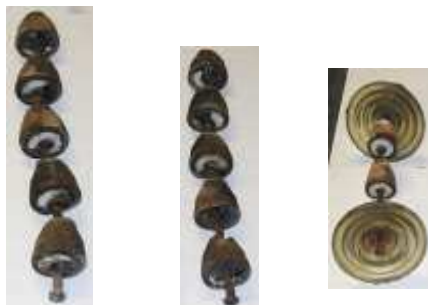
Photograph 1 – The severely damaged insulator strings in relation to structure 77QEVE35
