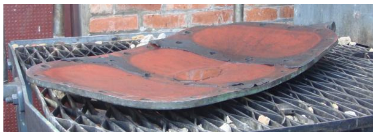
Photograph 2 – The damage to the Longcliffe 'A' teed Ashbourne 'A' 33kV circuit-breaker and the access door that was blasted off
