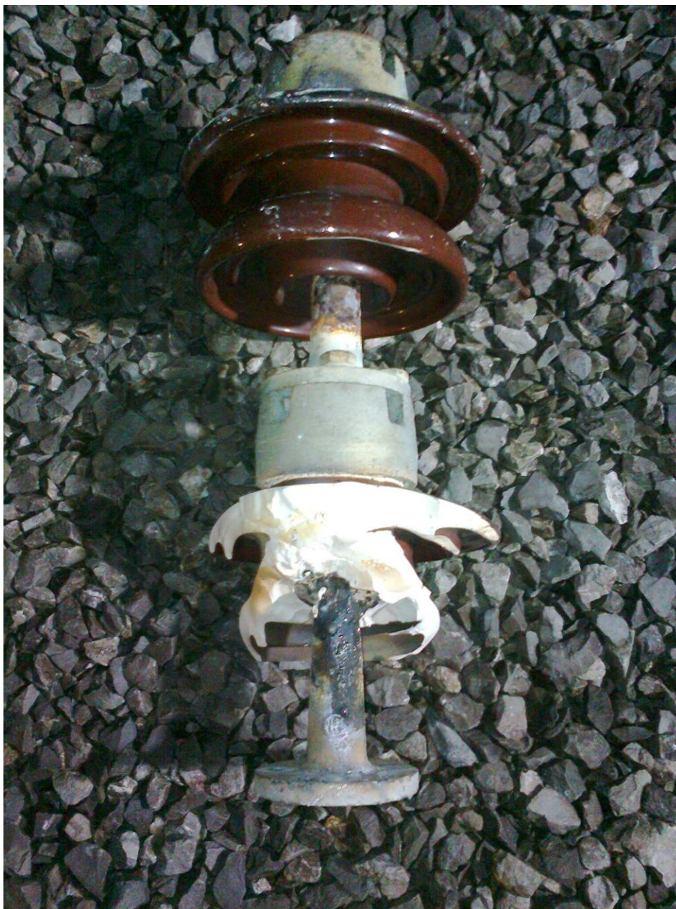
Photograph 2 – The irreparably damaged 33kV post-type insulator
