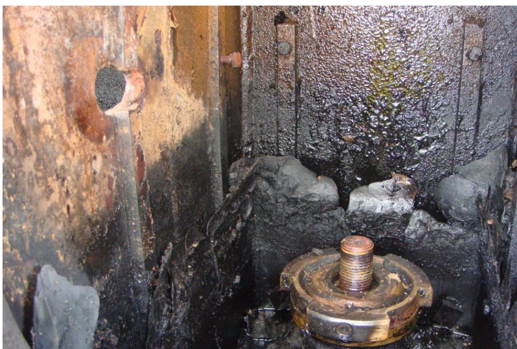
Photograph 4 – The arc damage within the interruption chamber
