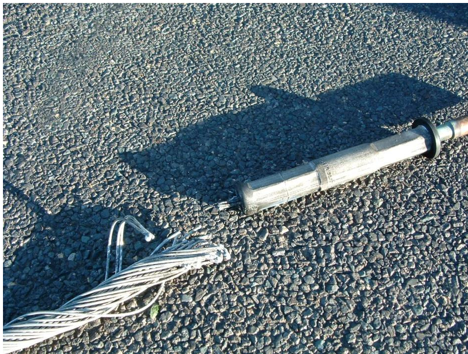
Photograph 2 The failed jumper connection in relation to the crimped lug
