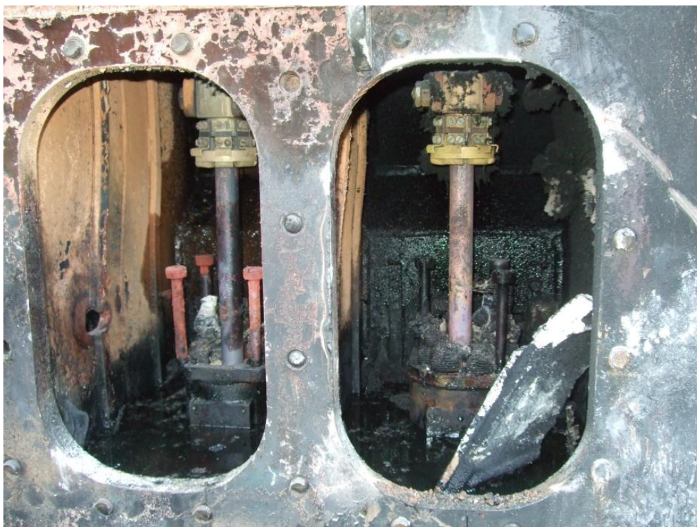
Photograph 3 – View of the damaged interruption chambers
