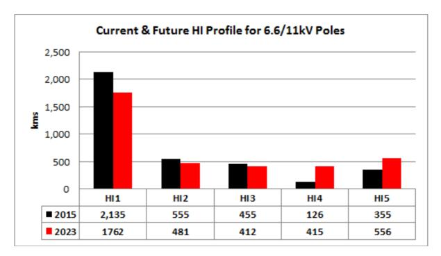
The key failure modes relating to poles are the failure of the pole due to decay and/or physical damage. This may be assessed visually (i.e. observed) or via a quantitative method to determine residual strength (i.e. measured). These Factors, given their strong correlation to residual strength and therefore probability of failure, have a relatively strong impact on HI when compared with other Asset Categories:
