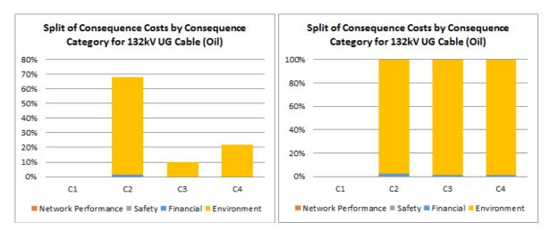
As shown earlier, 98% of the Reference Cost of Failure for this Asset Category is associated with the Environmental Cost of Failure. It therefore follows that once the Consequence Factors are applied, the overall Consequence of Failure will be driven by the Environmental Factors and specifically the proximity of the cable to a watercourse. The table below demonstrates this relationship:
