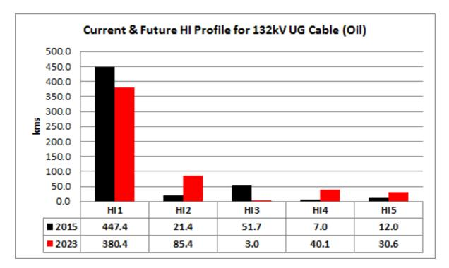
As described earlier, the key failure mode relating to oil-filled cables is the failure of the pressurising system and this is the more sensitive of the two Measured Condition Inputs applicable to this Asset Category. The table below demonstrates the correlation between HI Band and the "leakage" Measured Condition Input for two scenarios; (a) for younger cables defined in this instance as <50 years old and (b) for older cables, defined in this instance as  $\geq$ 50 years old:
