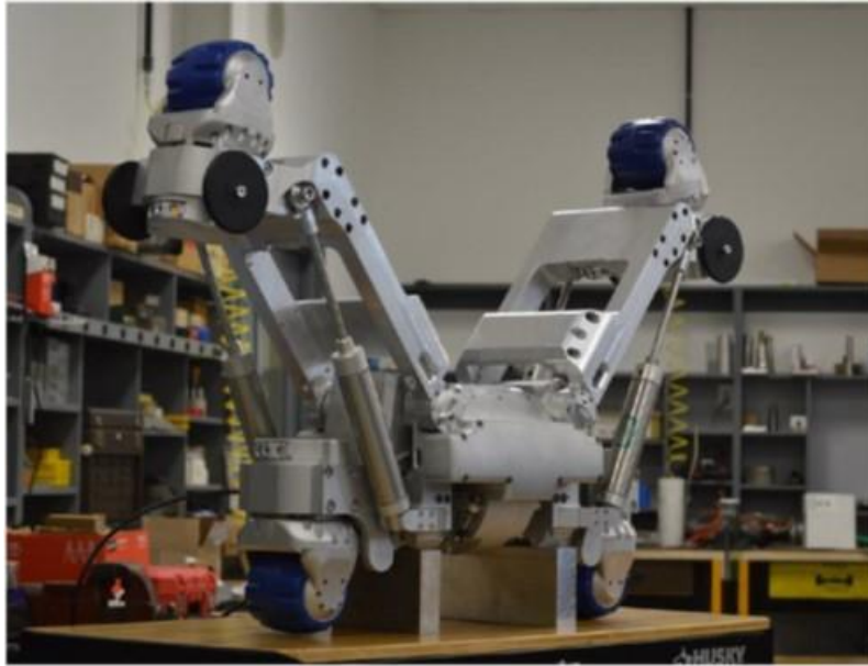
Figure 1 – Repair Robot Platform with the Wheels in the Driving Position
