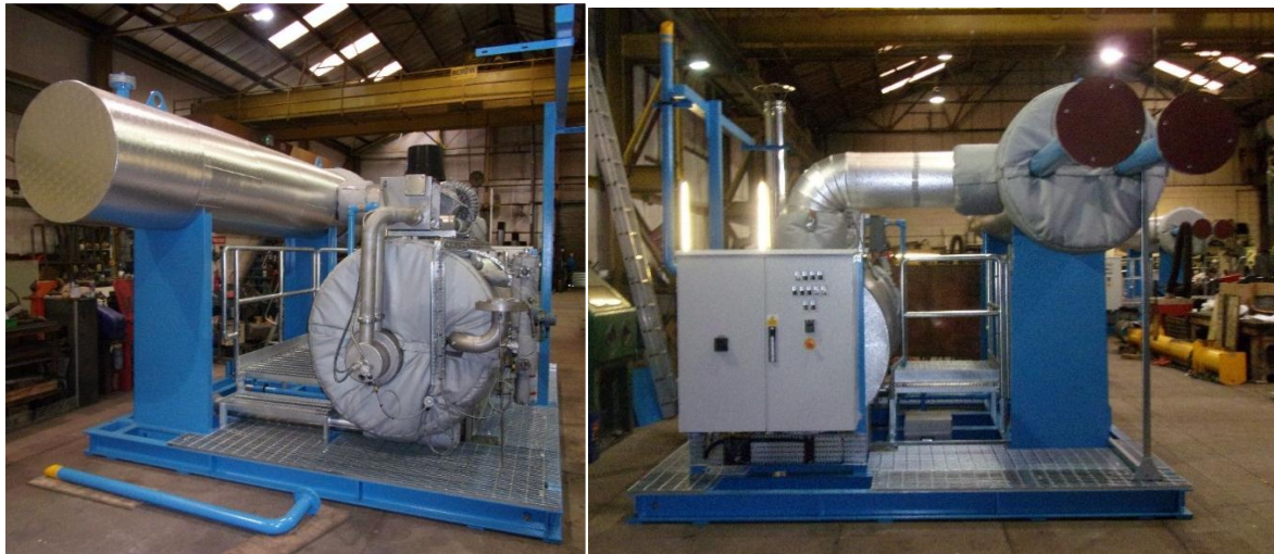
Figure 8. Little Burdon Proheat Units during factory testing
