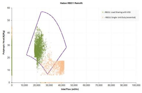
However, the RB211 DLE retrofit is only compliant with the CO emission limit specified in the IED at above 70% load and the diagram below shows the 70% load line. It can be seen that the vast majority of the data points fall outside of this range and therefore the RB211 retrofit is not considered BAT for Hatton.
