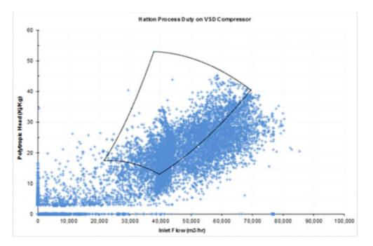
The operating points outside of the VSD envelope would need to be covered by another unit, i.e. the RB211 retrofit. Some of these points (green in the diagram below) would be covered by parallel operation and some of these points (orange in the diagram) below would be covered by single operation.
