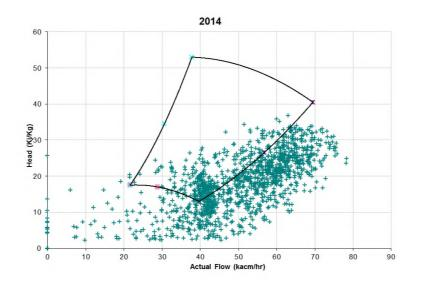
Based on the required duty, there would have been circa 600 and 1075 hours of operation that could not have been met at Hatton without additional compression in 2010 and 2014 respectively. The analysis excludes operating points associated with compressor start up. Given the combination of the normal operating duty being well in excess of 500 hours and the potential constraint costs, we conclude that the cost / benefit of installing one new unit is robust.
