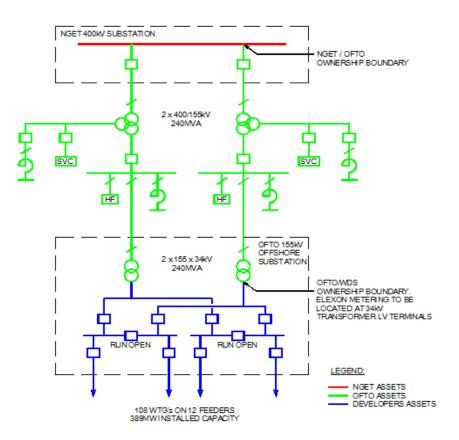
ANNEX B TO AMENDED STANDARD CONDITION E12–B1 (TRANSMISSION SYSTEM CIRCUIT) The transmission system is defined by the circuit diagram set out below.
