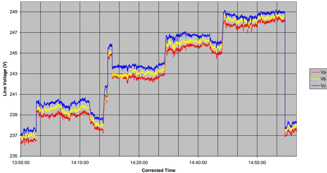
Figure 36: LV voltage as reactive power export is increased
