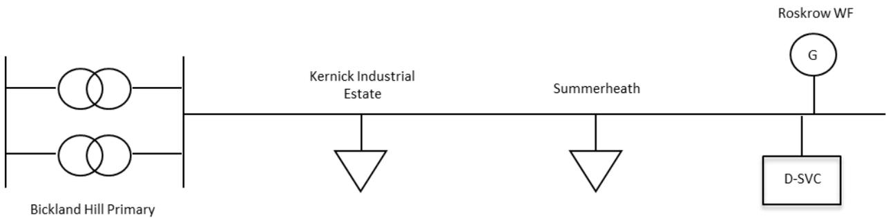
Figure 7: The 11kV feeder with monitoring locations
