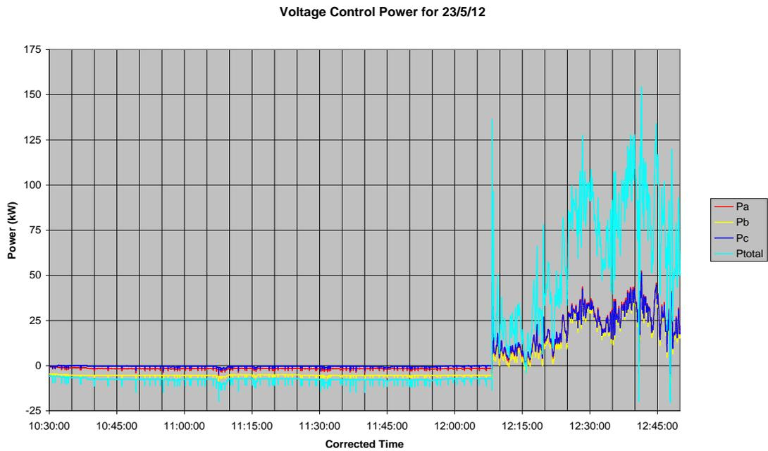
Figure 29: Real power output of the windfarm
