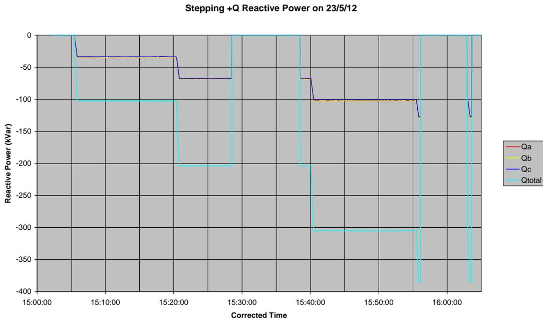
Figure 26: Reactive power output of the D-SVC
