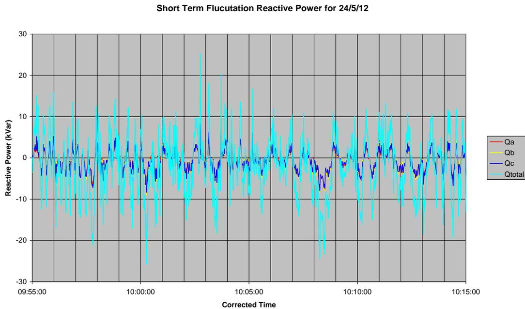
Figure 33: D-SVCs reactive power output in SFV mode
