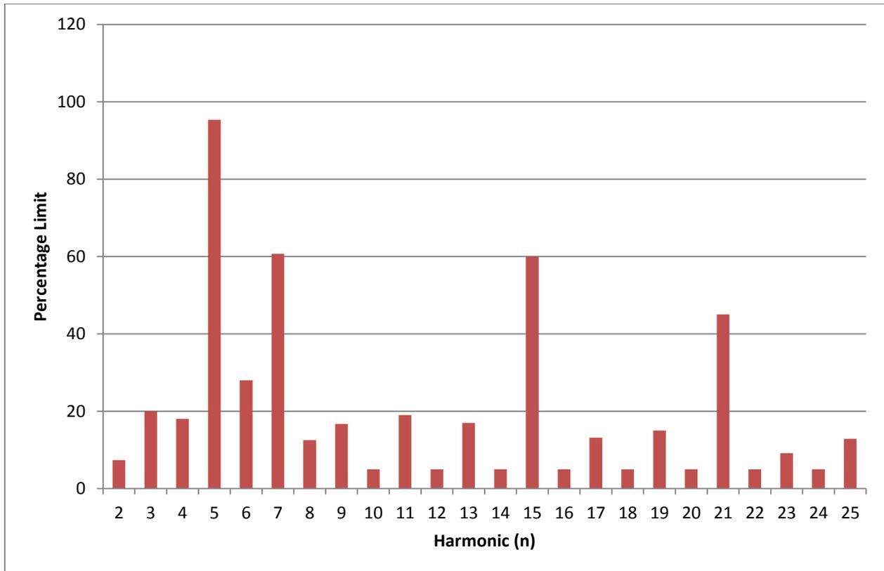
Figure 15: HV Harmonics measured by the Topas
