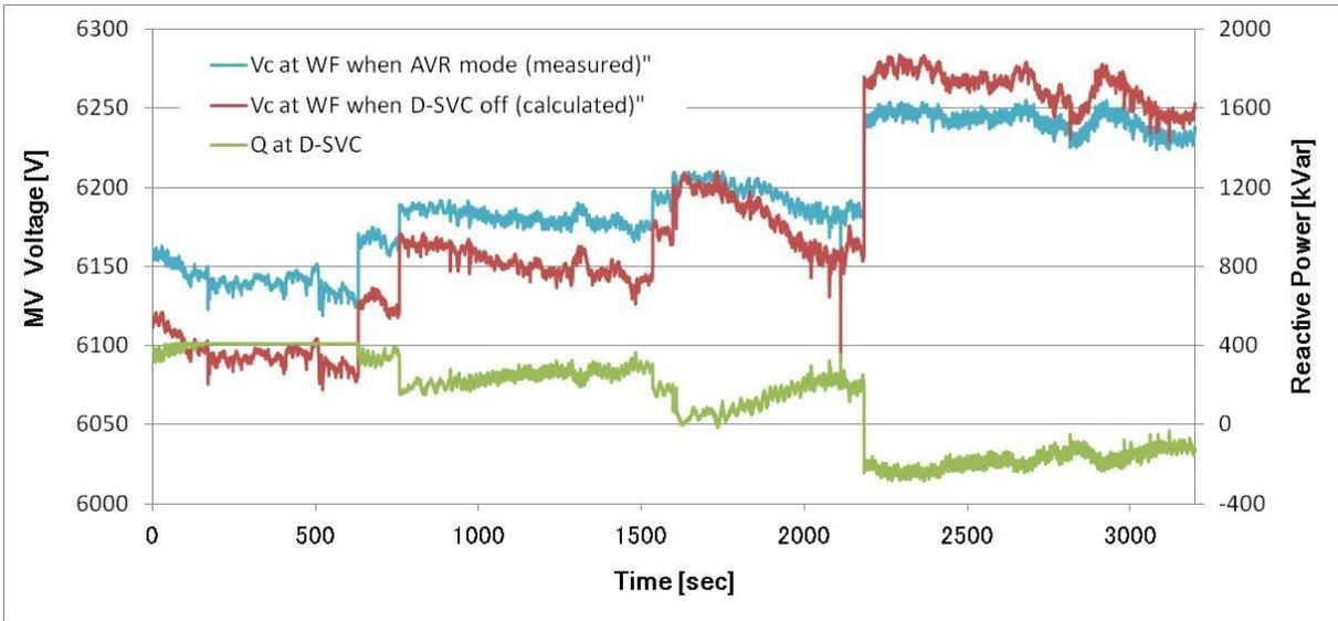
Figure 24: Calculated Vc at WF when D-SVC off
