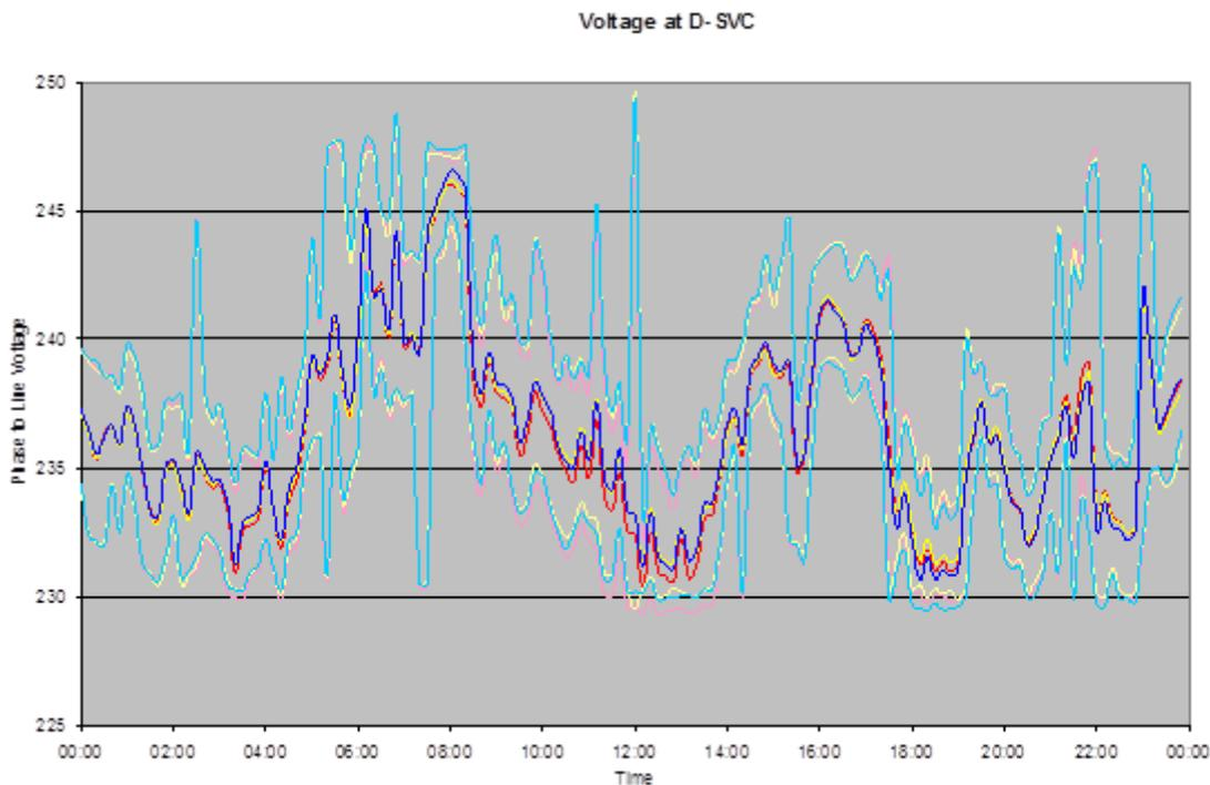
Figure 18: Voltage at the LV side of the D-SVC
