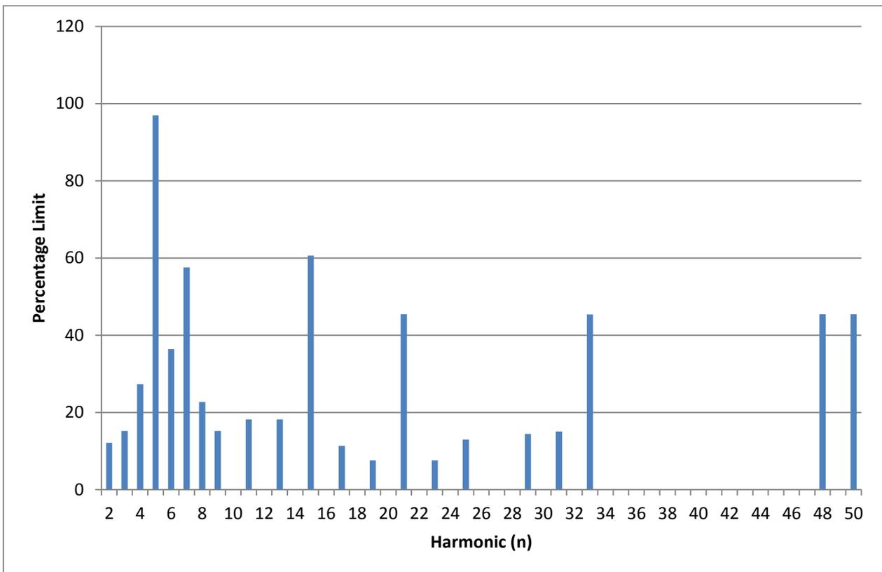
Figure 14: HV Harmonics measured by the PM7000
