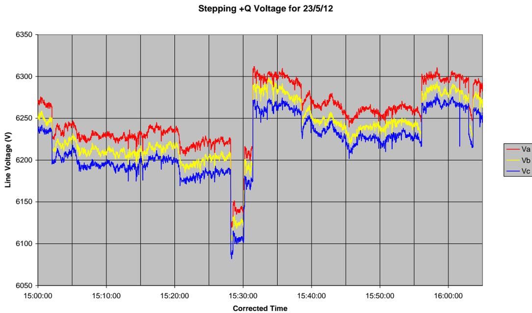
Figure 27: HV voltage while the D-SVC is absorbing reactive power
