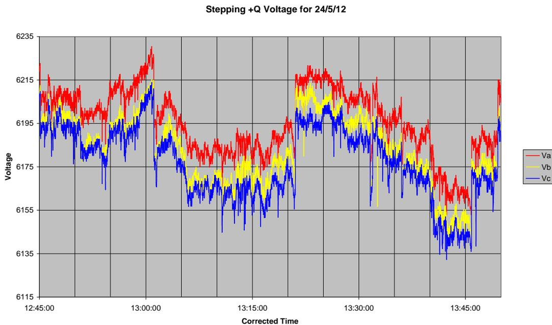
Figure 28: HV Voltage while reactive power is being absorbed
