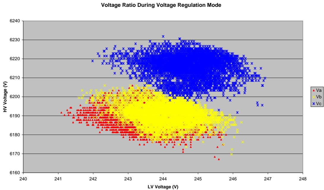
Figure 35: Voltage ration with the D-SVC operating in AVR mode
