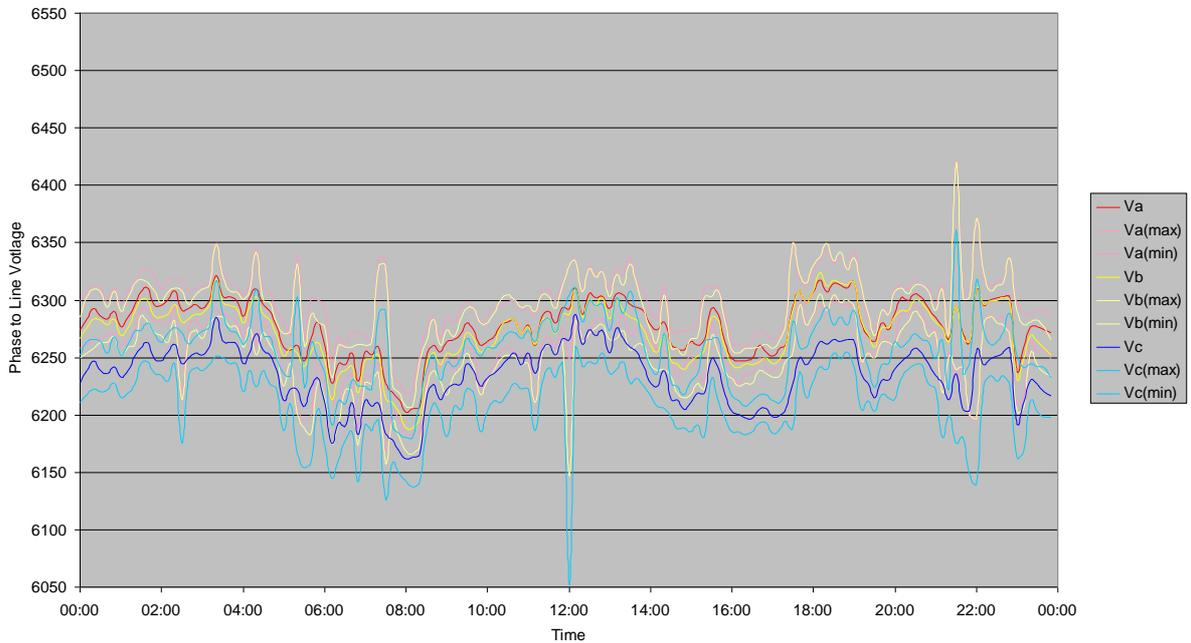
Figure 19: Typical HV voltage profile with the D-SVC running
