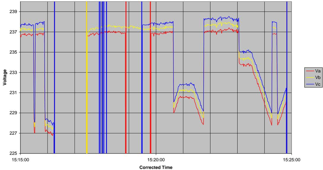
Figure 10: LV voltage during reduction in voltage
