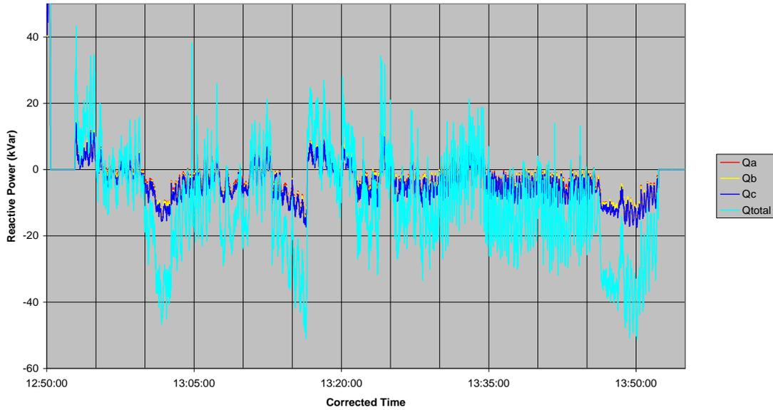
Figure 31: D-SVC reactive power output in ARV mode
