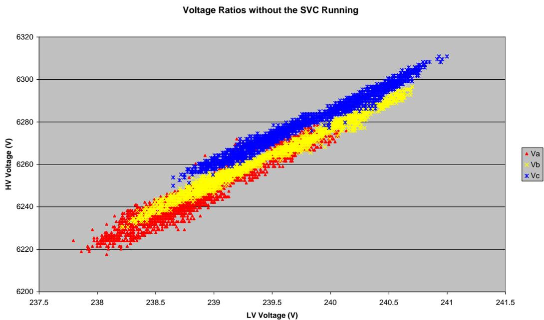
Figure 34: Voltage ratio without the D-SVC running
