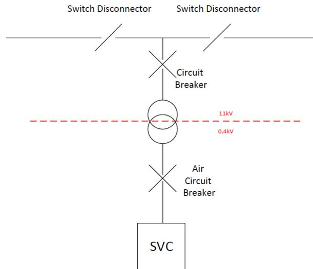
Figure 3: Signal Line Diagram of equipment on site
