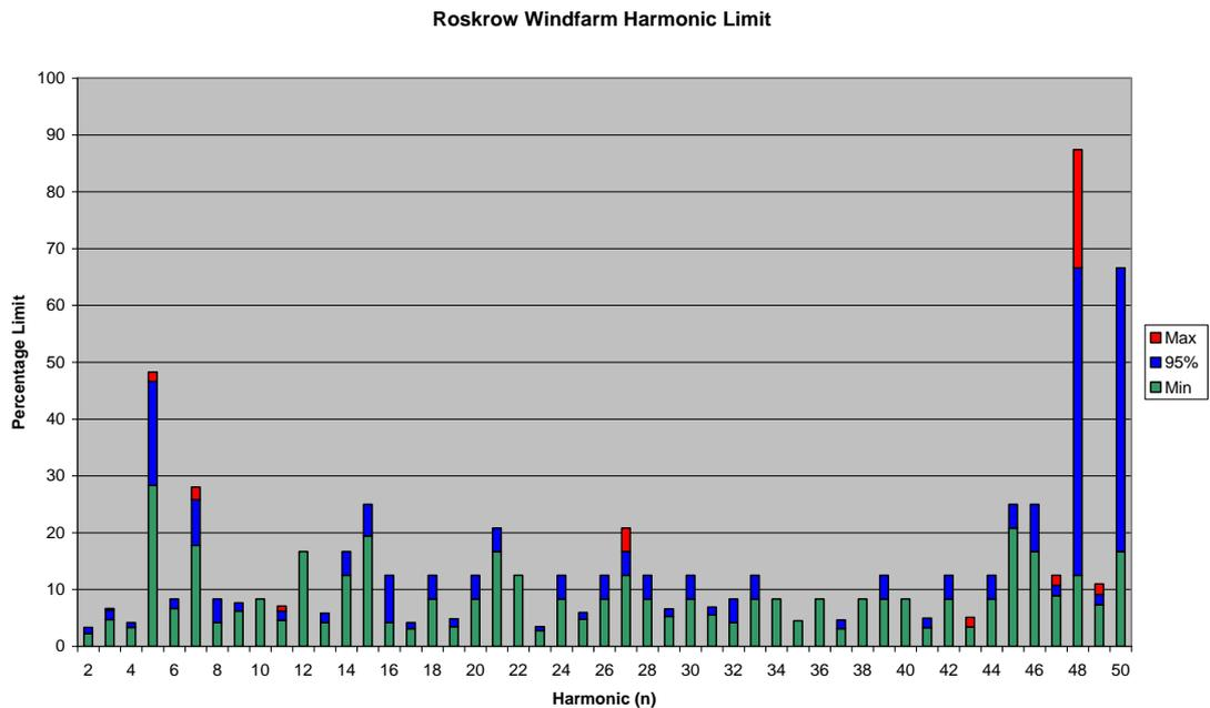
Figure 13: Harmonics on the HV side of the transformer
