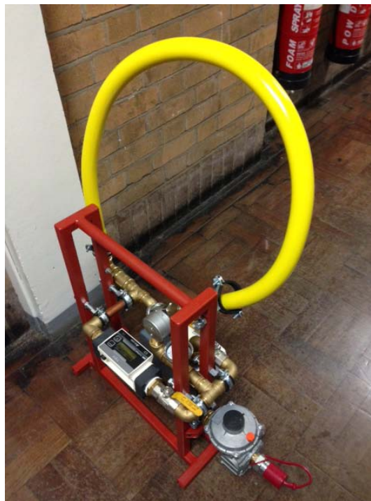
FIG 8 – Meter rig, for connection between testing kit and customer property
