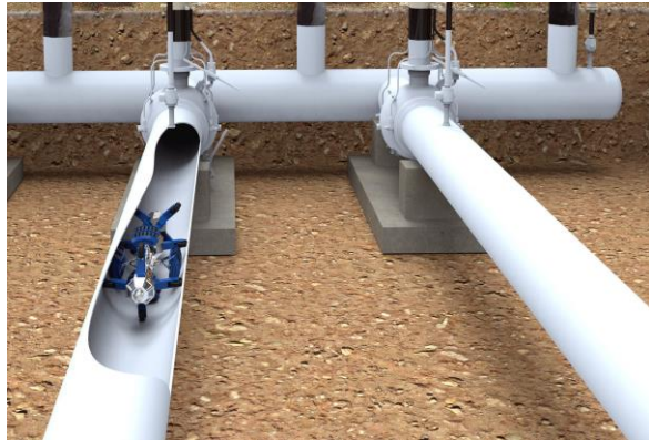
Fig 1: Innovative Robot within pipework.
