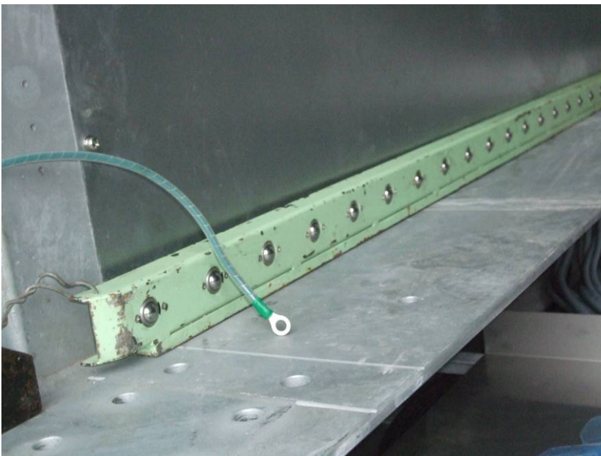
Figure 14 - Ball bearings reduce friction
