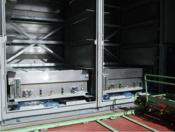
Figure 15 - Track allows quick repositioning of insertion tool
